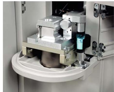
**The zero blank loading head is designed for consistent wafer loading along with pins, chips, and powders.**
